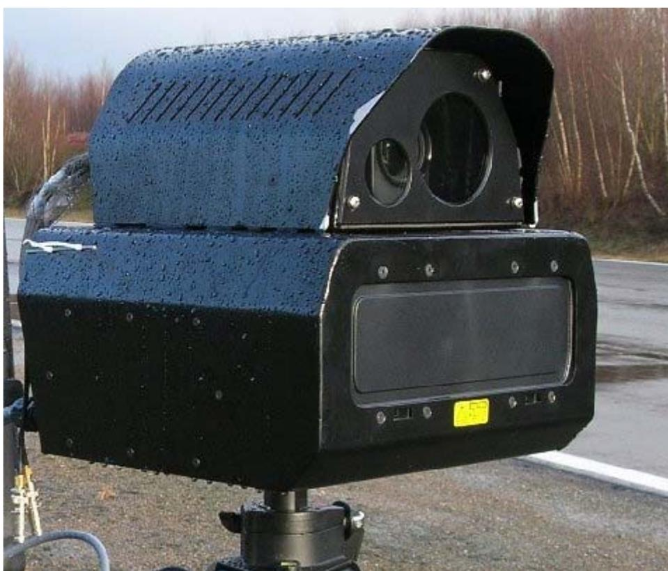
**Figure 2 - AGD / Redflex portable safety camera**
