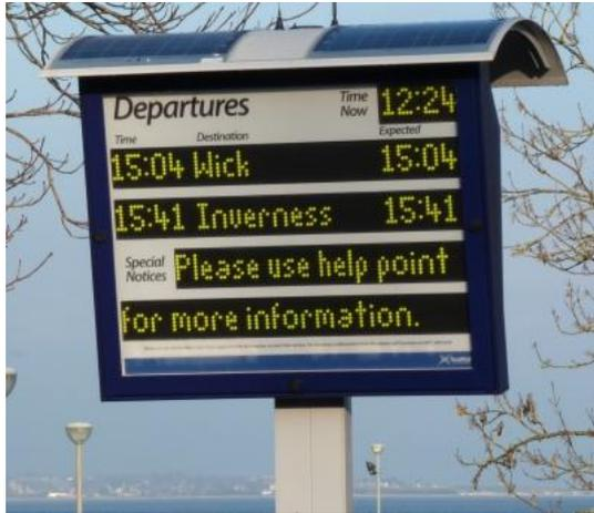
*Low cost solar powered display by Nexus Alpha Low Power Systems*
